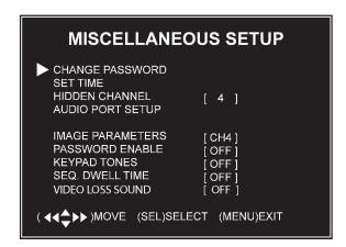
The default password is set to "111111". You may change the password, but be sure to write it down and keep it in a safe place so you do not forget the new password. To change the password:
